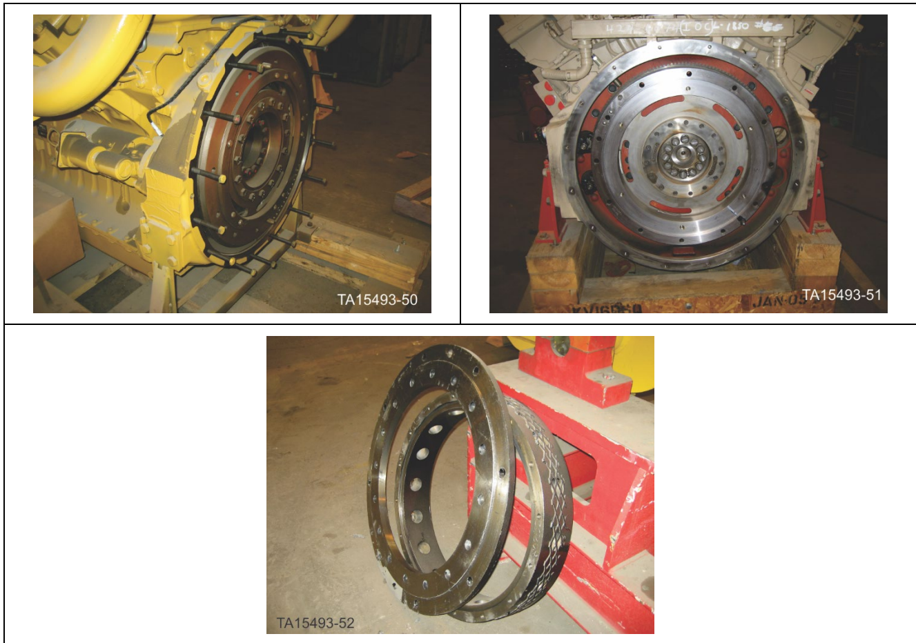
Figure 254. Clean All Mounting Faces and Shoulders
