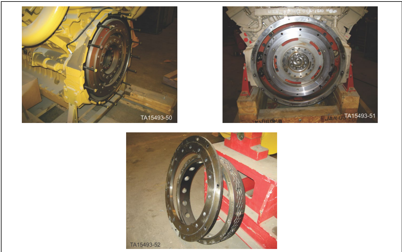
Figure 146. Clean all mounting faces and shoulders
