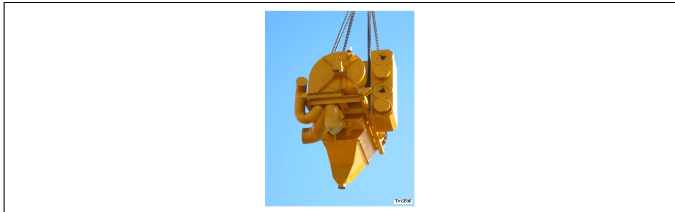
Figure 62. Hoisting of KLENZ™ and blower assembly
