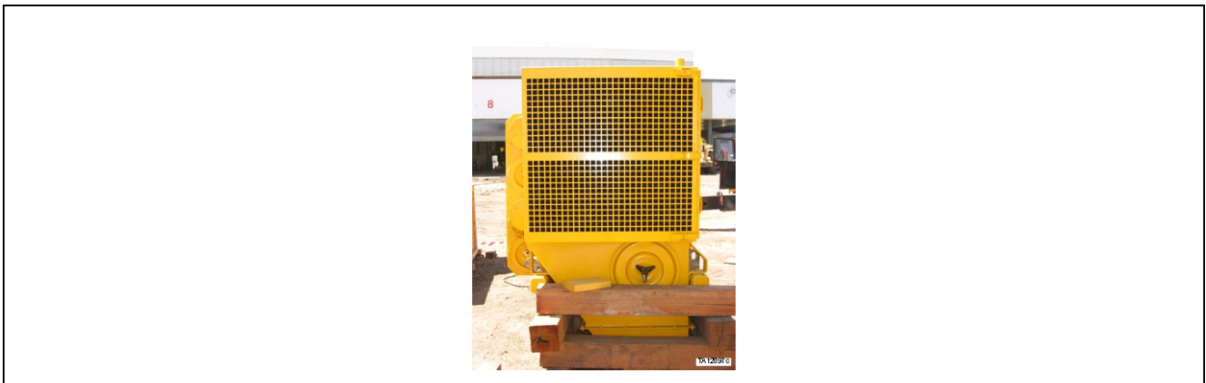
Figure 65. KLENZ™ and blower assembly supported by cribbing - 3 of 3
