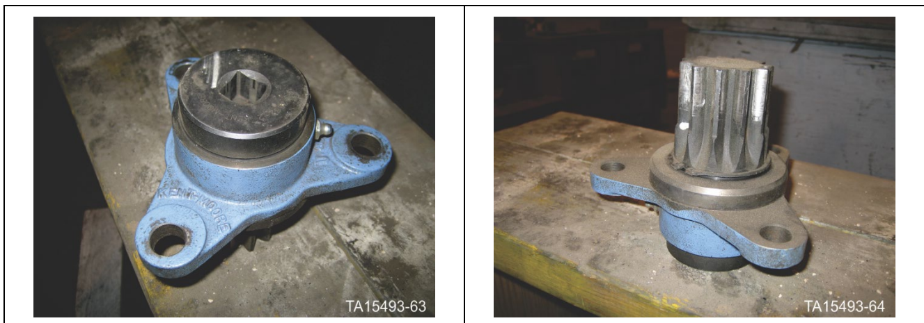
Figure 264. The engine rotation tool must be removed from the engine after each use.
