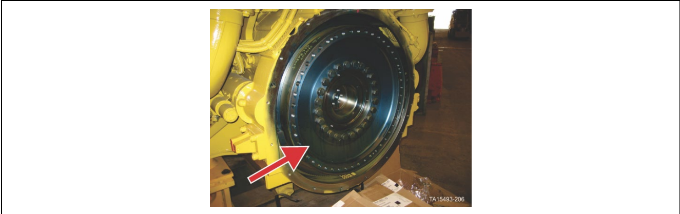
Figure 160. Measurement of radial runout of engine flywheel - Tier 2 DD/MTU
