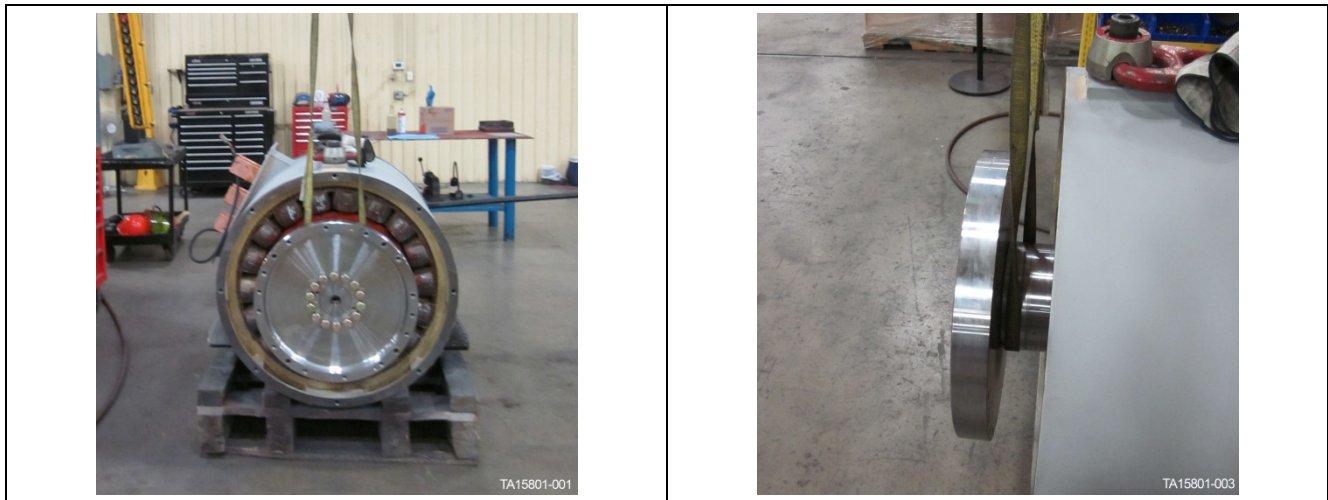
Figure 125. Lifting strap located on Drive End
