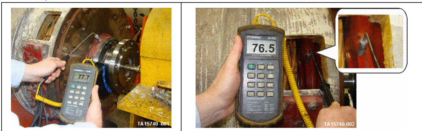
Figure 310. Typical temperature bearing testing
