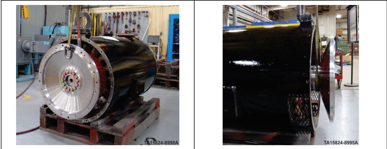
Figure 236. Lifting strap located on drive end
