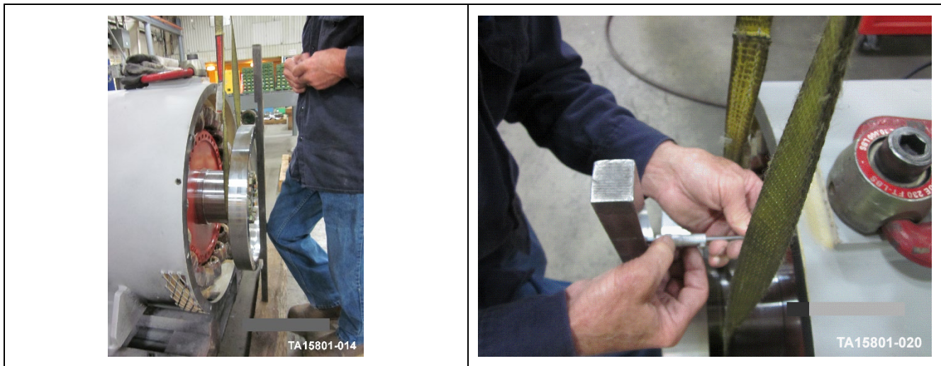
Figure 134. Measurement between a straight edge and generator stator
