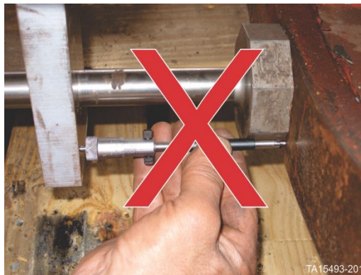
Figure 244. Do not measure between endplay brace as it is most likely not a straight edge
