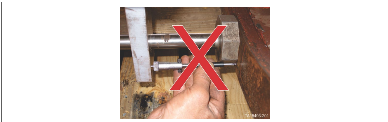
Figure 133. Do not measure between endplay brace as it is most likely not a straight edge
