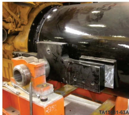
Figure 294. Join motor and generator together
