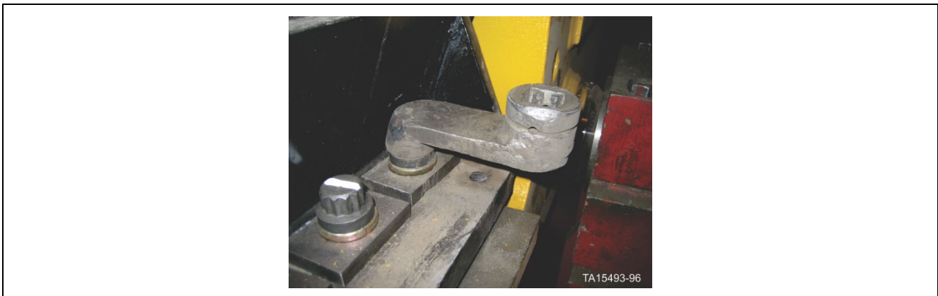
Figure 193. Offset adapter may be required to torque the bolts on the generator
