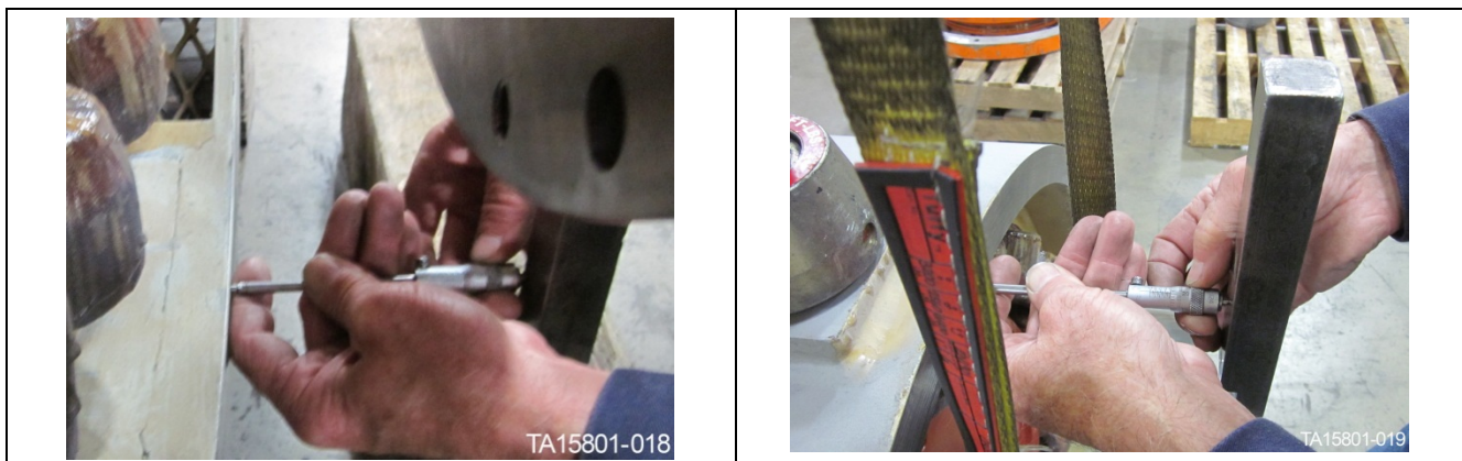
Figure 135. Measure "adapter to stator dimension" between face of rotor and face of generator pole ring
